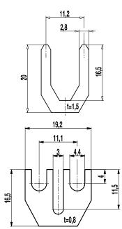
Jumper 307-V is designed for the tab/screw connectors of series 307-PCF and 3070-PCM. By pushing them into to the tubular rivets from the top, it connects two adjacent poles to an impeccable electrical contact. This jumper cannot be used in combination with the cover caps.
